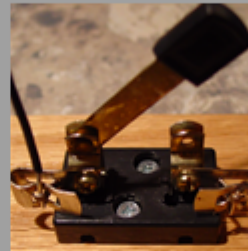
Also called a Single Pole Single Throw switch (SPST).
